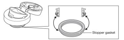
Slowly remove the stopper gasket while holding its edge. When attaching the stopper gasket, make sure to fit it completely in the proper direction.
