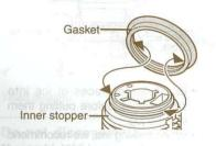
Attach the gasket fully and securely
